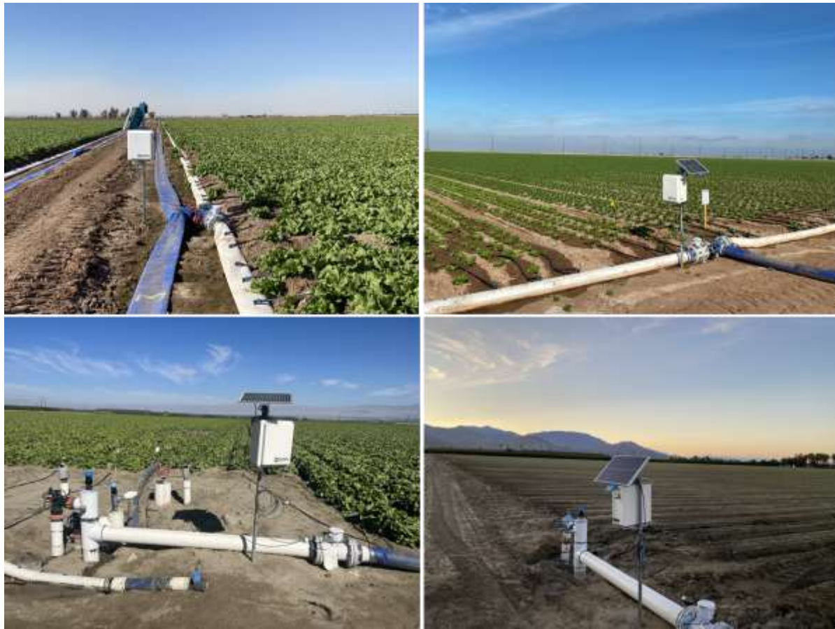
Fig. 1. A demonstration of the trial fields. The water applied was measured using magnetic flowmeter attached to datalogger. The data of water applied was automatically imported and analyzed by CM tool.
