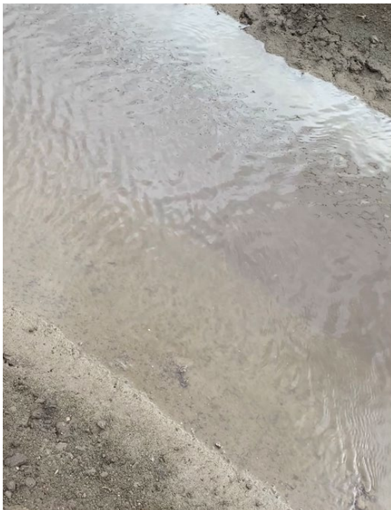
Figure 2. Runoff from a brassica field that was sprinkler irrigated with water treated with PAM using the well applicator.
