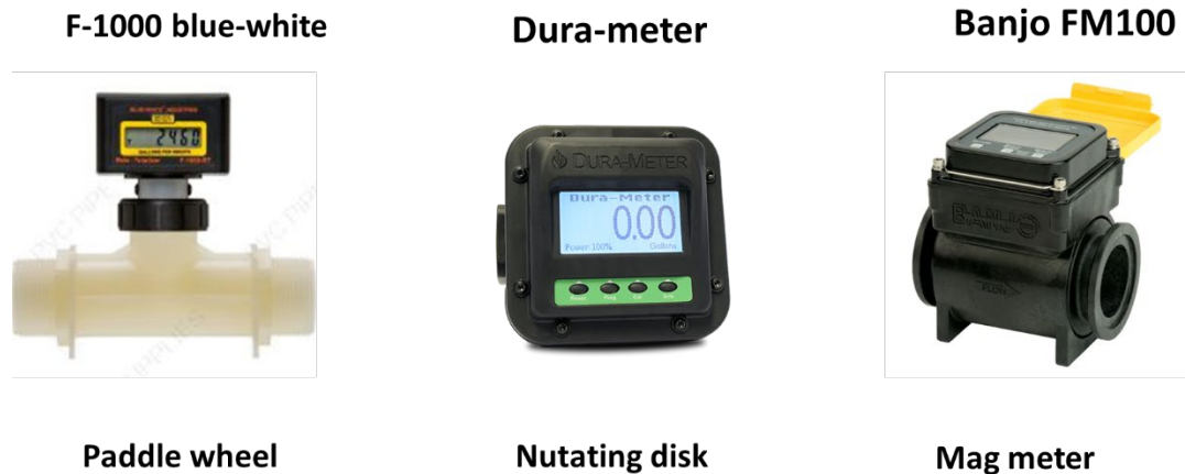
Figure 1. Three models of flowmeters that use different mechanisms for measuring flow were evaluated for accuracy in measuring the volume of fertilizer pumped from a tank.
