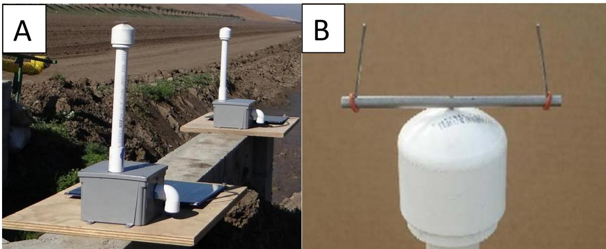
**Figure 1.** Spore trap system to detect *Peronospora effusa*, the causal agent of spinach downy mildew, respectively. **A)** Example of two spore traps in operation. **B)** Spore trap head with rotating arm and removable stainless-steel rods coated with grease for spore adhesion.
