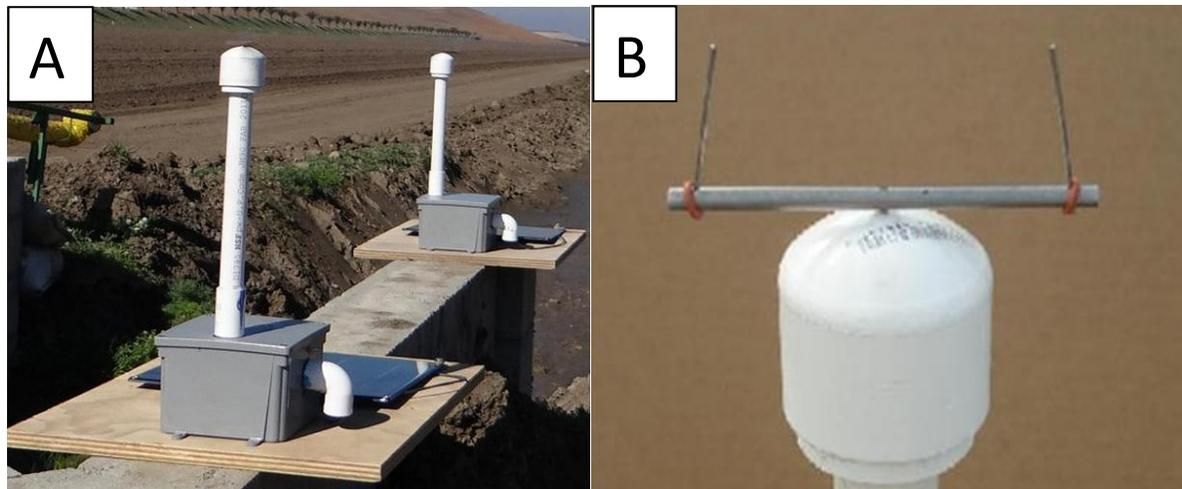
**Figure 1.** Spore trap system to detect *Bremia lactucae* and *Peronospora effusa*, the causal agents of lettuce and spinach downy mildew, respectively, in the Salinas Valley, California. A) Two spore traps in operation south of King City, CA. B) Spore trap head with rotating arm and removable stainless steel rods.
