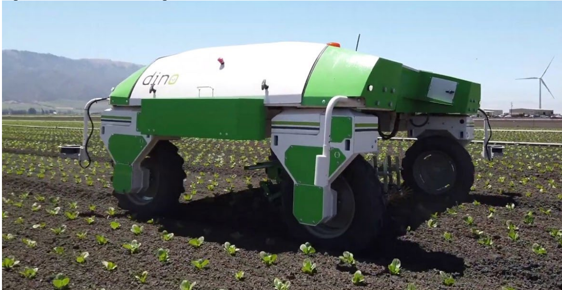
Figure 1. NAÏO Dino autonomous cultivator equipped with finger weeders.
