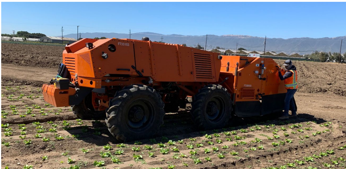
Figure 2. Farmwise Titan autonomous cultivator equipped with paired cultivator knives.
