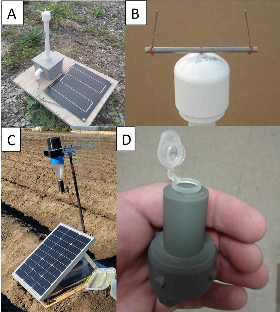
**Figure 1.** Two spore trap systems to detect airborne *Peronospora effusa* and *Bremia lactucae*. **A)** Example of a spore trap in operation. **B)** Impaction spore trap head with rotating arm and removable stainless-steel rods coated with grease for spore adhesion. **C)** A cyclone spore trap from Root Applied Sciences. **D)** In the cyclone spore trap, the spores of the pathogen and similar sized particles drop through a center of a cyclone, into the microfuge tube shown.
