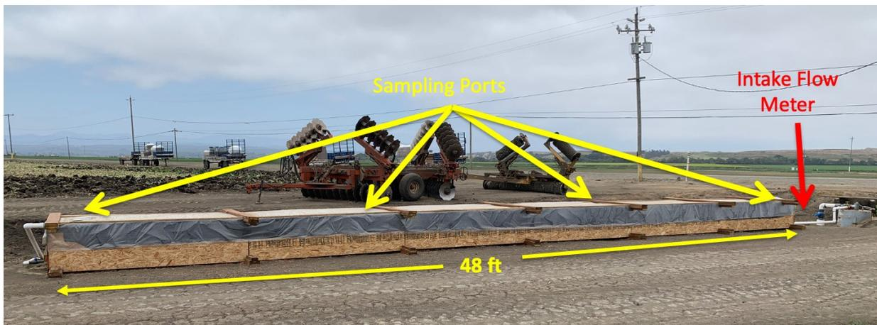
Figure 1. Photo of the bioreactor system installed at the Odello Ranch in Salinas, CA.
