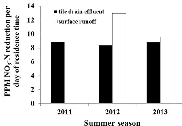
Fig. 1. Mean reduction in NO<sub>3</sub>-N concentration per day of bioreactor residence time; values for tile drain effluent are averaged across sites 1 and 2.
