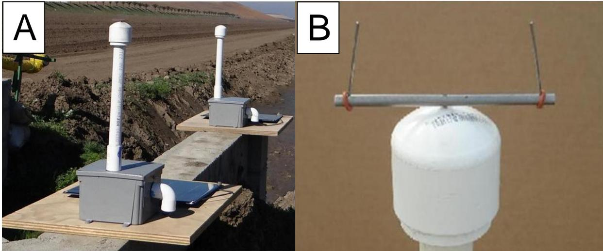
Figure 2. Spore trap system to detect *Peronospora effusa*, the causal agent of spinach downy mildew in the Salinas Valley, California. A) Two spore traps in operation south of King City, CA. B) Spore trap head with rotating arm and removable stainless steel rods.
