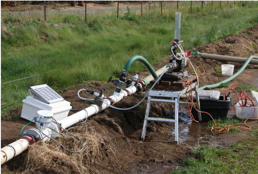
**Figure 3.** Manifold used to mix well water, sprinkler runoff and pesticide in the simulation trials.
