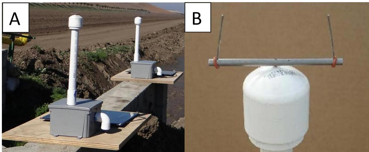
**Figure 1.** Spore trap system to detect *Bremia lactucae* and *Peronospora effusa*, the causal agents of lettuce and spinach downy mildew, respectively. **A)** Two spore traps in operation south of King City, CA. **B)** Spore trap head with rotating arm and removable stainless-steel rods.
