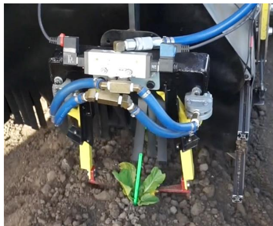
Figure 7. Photograph showing the UC Davis robotic hoe automatically avoiding the lettuce plant containing the biodegradable, machine readable plant label.
