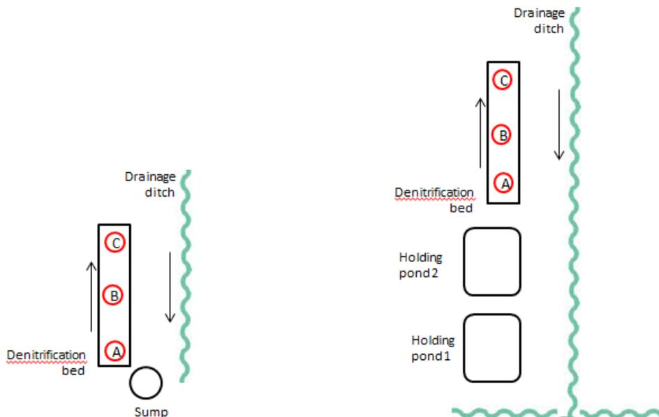
**Figure 2. Placement of chambers at each field site, DBR 2 (left) and DBR 3 (right). Chamber A was located within the first six feet of the bioreactor near the *inlet*, chamber B about 18 feet down (*middle*), and chamber C over 30 feet down near the *outlet*.**
