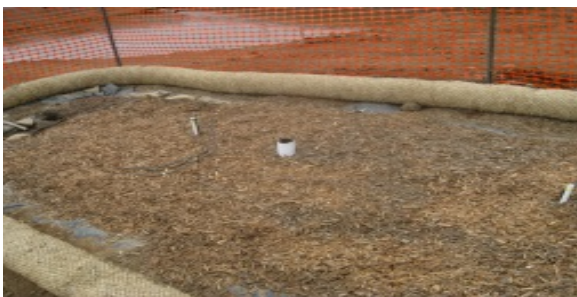
Figure 1. (a) Location of baffles and monitoring wells, according to the dimensions of DBR 3; and (b) view of the bed with two narrow PVC monitoring wells tops sticking out several inches above the surface and one larger pipe used by the UC Cooperative Extension also apparent. The inlet pipe is to the far left of the photograph.
