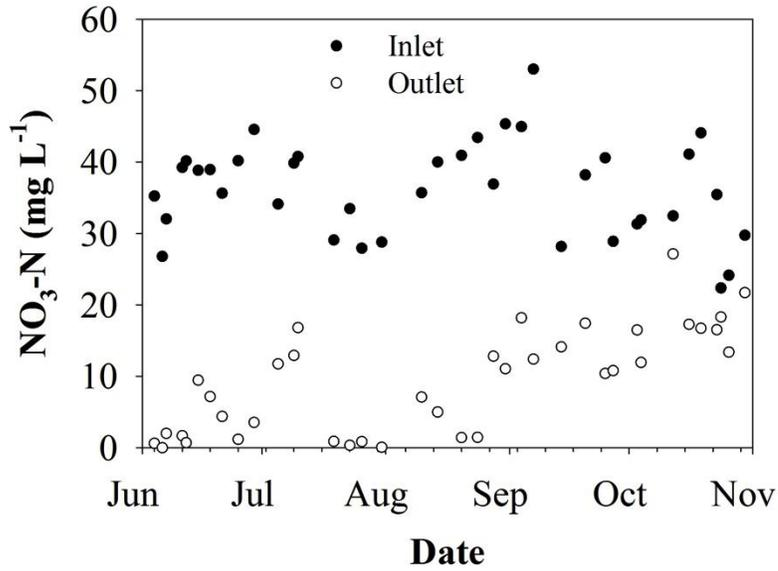
Figure 2. Reduction of water  $\text{NO}_3\text{-N}$  concentration during treatment in the denitrification bioreactor treating surface runoff (site 3).
