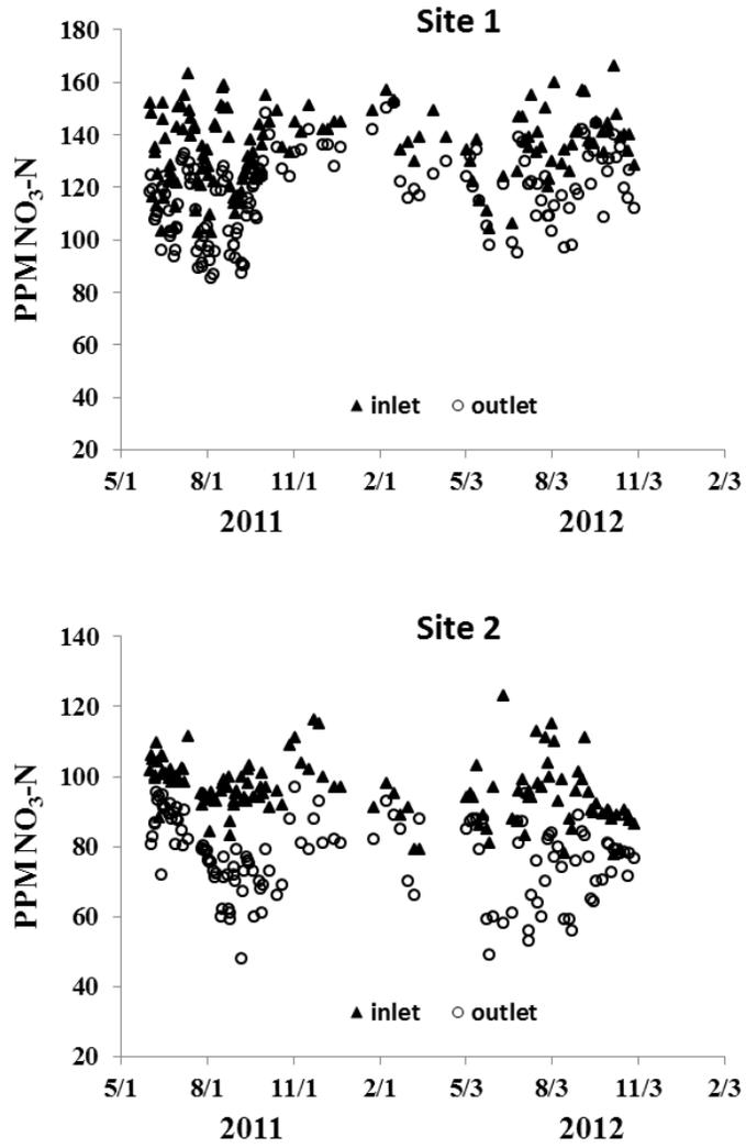
Figure 1. Reduction of water NO<sub>3</sub>-N concentration during treatment in the denitrification bioreactors treating tile drain effluent.
