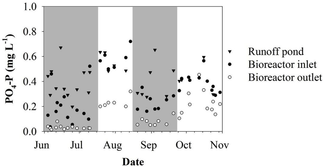
Figure 3. Effect of alum and bioreactor treatment on  $\text{PO}_4\text{-P}$  concentration of surface runoff water (site 3). Shaded areas represent periods during which alum was injected.
