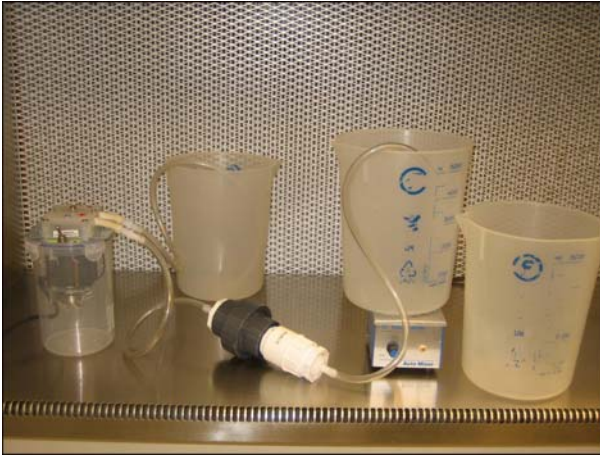
Figure 3. Laboratory setup to evaluate capture efficiency in single-pass filtration with Modified Moore Swab
